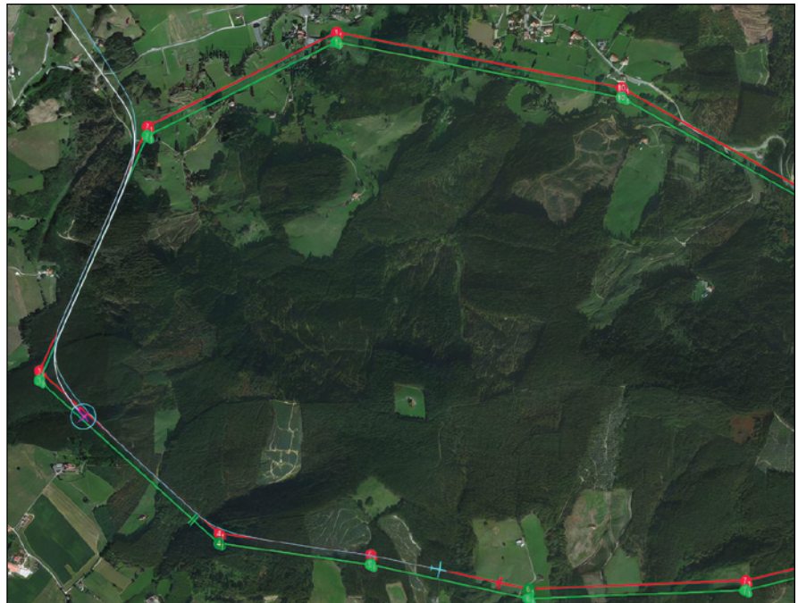
Two UAVs executing the same flight plan and being commanded from the same ground control station software. (Image: UAV Navigation-Grupo Oesía)
